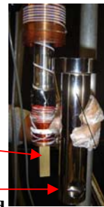
Radiant Heat Shield
